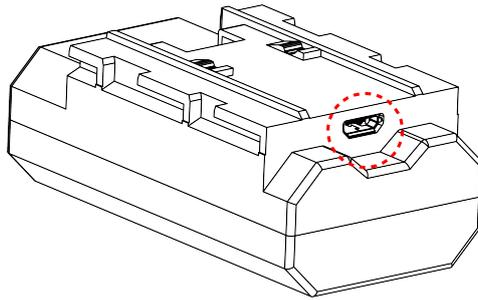
Charge the battery with the USB cable that we provided and a normal USB power adapter. A red light will flash while the battery is charging. When the battery is fully charged, the light will keep on.
