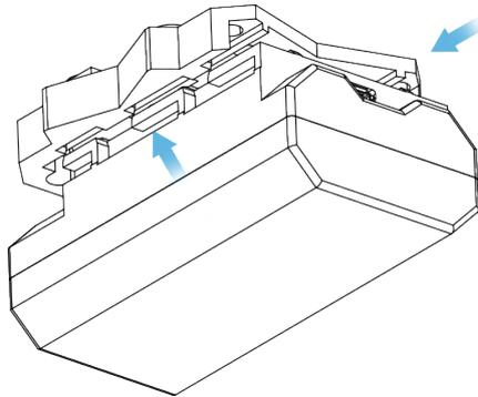
Put the battery in the socket and push it backward still it locked
